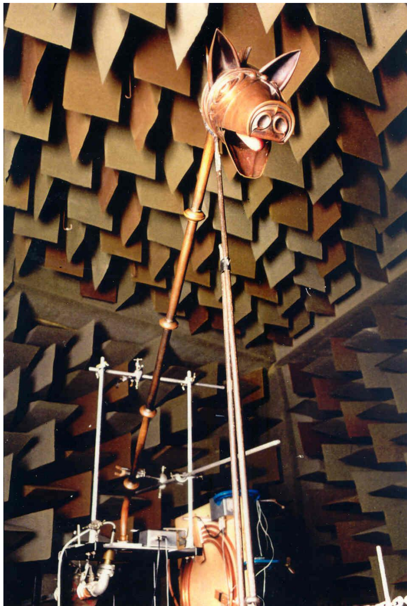
Measuring input impedance of prototype University of Edinburgh (1992)
